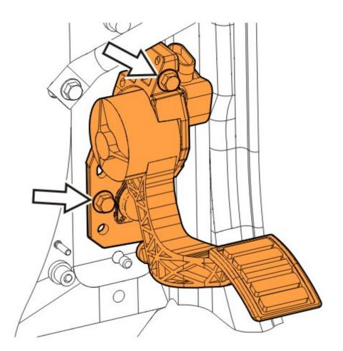
Install replacement accelerator pedal and tighten fasteners to 24 ± 4 Nm (18 ± 3 ft-lb).
