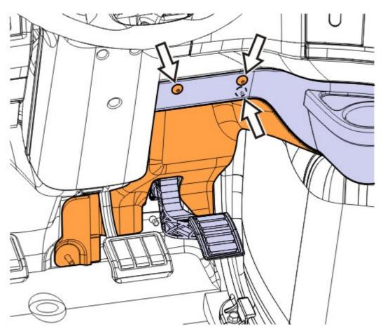
Remove the upper fasteners from both lower right dash panels and remove the panels.
