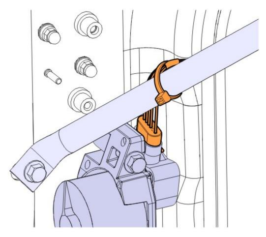
Disconnect the throttle position sensor harness and cut plastic cable tie from support bracket.
