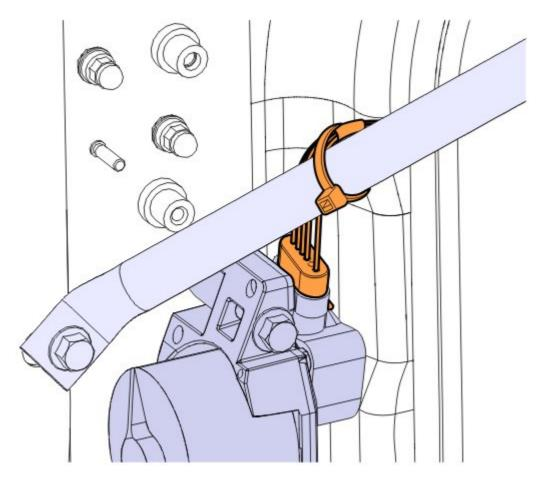
For trucks in production after 09/23/2013, connect the throttle position sensor harness and secure harness with cable tie as shown.
