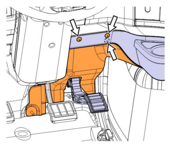
Install lower right dash panel fasteners.
