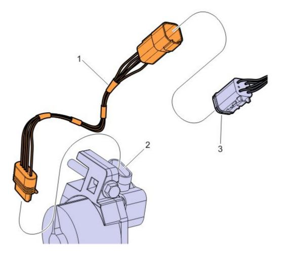
Note: Trucks in production before 09/23/2013 will require a jumper harness and conversion kit. Reference TPI 271–012PB for part numbers.
