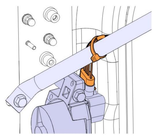
Secure harness with cable tie as shown.
