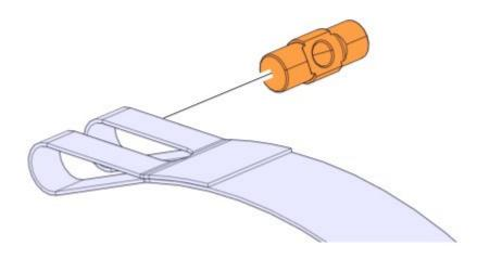
22 Install the tensioning band.
