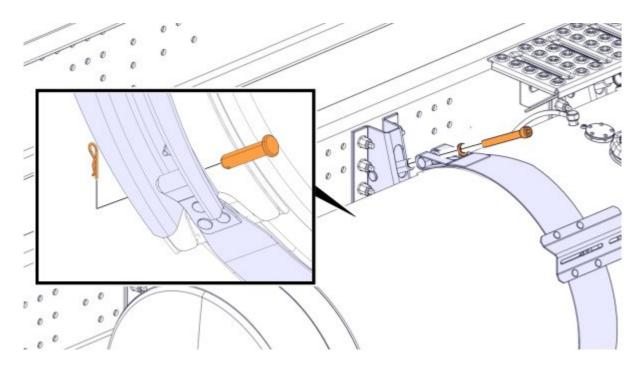
Remove the tensioning band.
