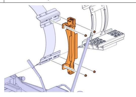
Remove the screw and washer.
