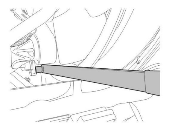
With the belt tensioner compressed, install the replacement fan and water pump drive belt over the pulleys. Relax the tensioner against the drive belt.
