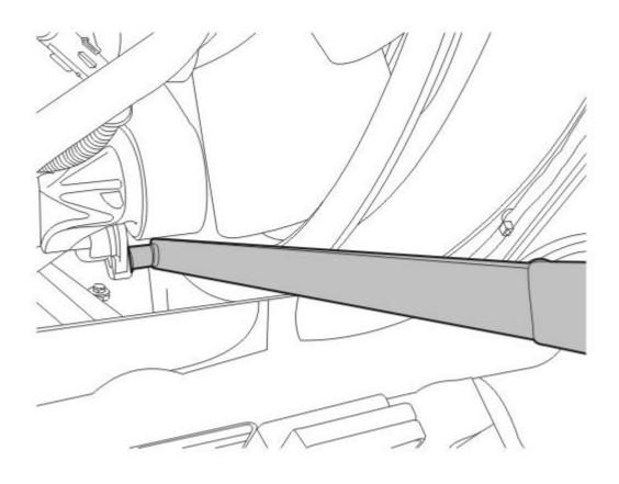
Pry the belt tensioner away from the fan and water pump drive belt and remove the belt.
