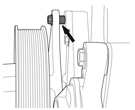
Loosen the fan hub mounting fasteners so that the hub can be moved forward to allow the belt to pass between the balancer and the fan hub.
