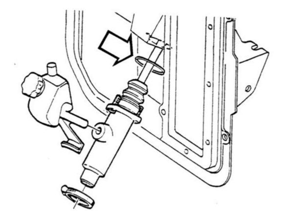
Install reservoir on the master cylinder and secure with band clamp. Torque band clamp to 3 Nm (26 in-lb).
