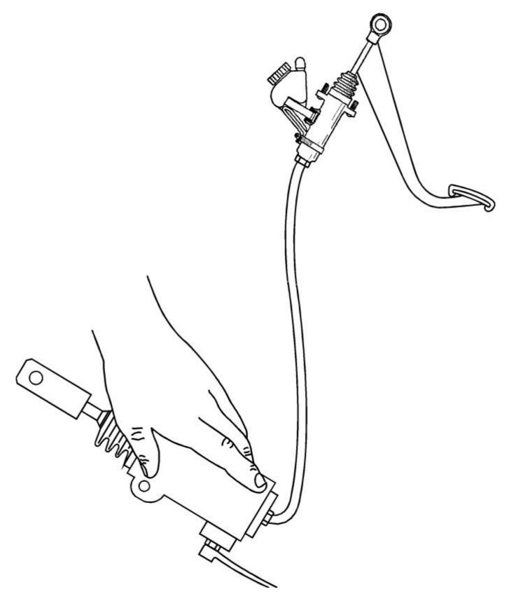
Open the bleed screw and connect the bleed tool. Clean the reservoir filler cap area and remove the cap. Hold the slave cylinder with the bleeder screw at the lowest point and turn the bleed pump on.
