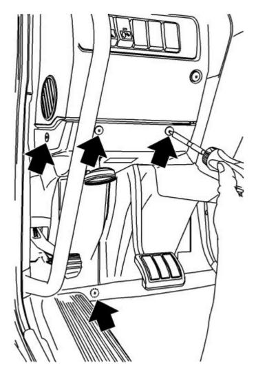
Install the left panel. Install the diagnostic connector. Install the heater hose, three torx screws and the plastic nut.
