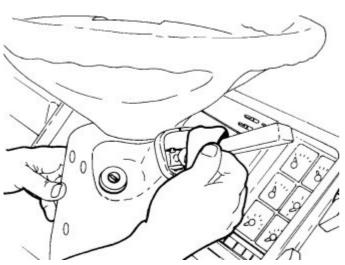
Put the dust covers in place on the turn signal and windshield wiper switches.
