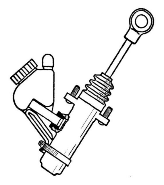
Remove the band clamp holding the reservoir. Remove the reservoir by pulling the reservoir out of the rubber seal.
