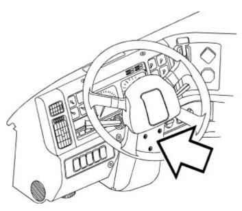
Remove the cover on the steering wheel column by removing the ignition key and the three torx screws.
