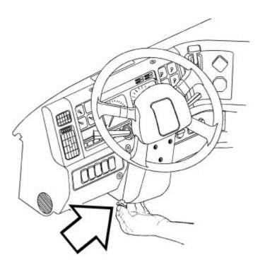
Remove the two clips at the bottom of the steering column. Remove the cover over the lower steering column by removing the plastic rivets.
