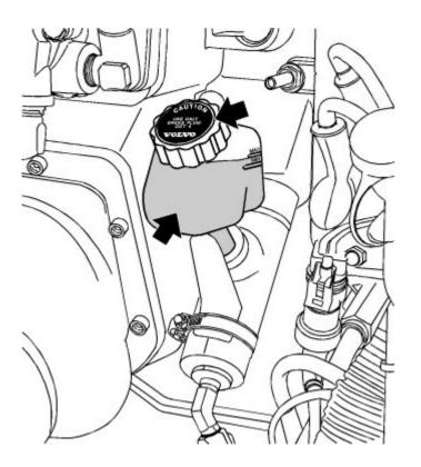
Stop bleeding when the fluid is at the minimum level indicated on the side of the reservoir. Close the bleeder screw. Torque bleed screw to 10 Nm (7 ft-lb).
