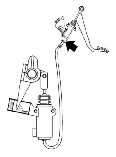
Tighten 45 degree fitting to proper angle and install the fluid line with a new O-ring. Torque fluid line to  $40 \pm 5$  Nm ( $30 \pm 4$  ft-lb).
