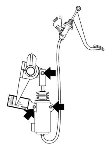
Remove the two slave cylinder mounting bolts and the clevis pin.
