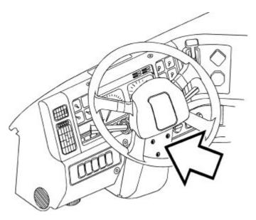
Install the upper cover on the steering column with three torx screws.
