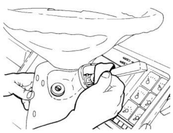
Pull the dust covers back on the turn signal and windshield wiper stalks.
