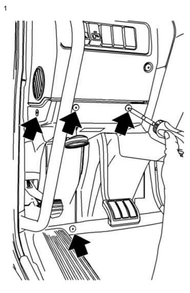
Pull the floor mat back and remove the plastic nuts fastening the left panel. Remove the three torx screws and the diagnostic connector. Pull the heater hose out of cover and remove the cover.
