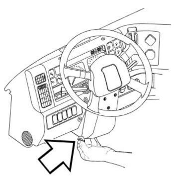
Install the two clips at the bottom of the steering column cover.
