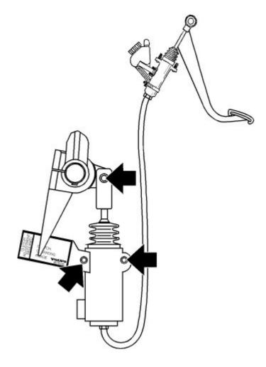
Install the clevis pin and the slave cylinder mounting bolts with the operating range tag. Torque the mounting bolts to 35 Nm (26 ft-lb).
