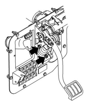
Install master cylinder. Make sure the O-ring is fitted around the neck of the master cylinder before the cylinder is inserted into the pedal plate assembly. Press the clutch pedal down to access the two mounting bolts. Torque mounting bolts to  $24 \pm 4$  Nm ( $18 \pm 3$  ft-lb).
