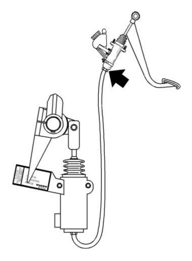
Remove the fluid line and remove the master cylinder from the pedal plate assembly.
