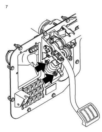
Remove the clutch pedal return spring to access the two master cylinder mounting bolts.
