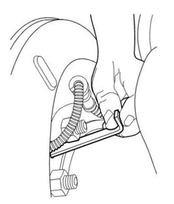
Slide the notched end of the sensor adjustment tool J-42942 through the opening in the brake spider until it rests against the sensor (the tool will go in the hole at a slight angle).
