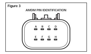
2. Connect the volt-ohm meter to the appropriate pins and measure the resistance. Coil resistance must be between 35 and 60 ohms.
