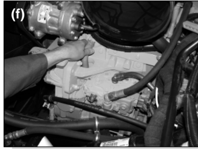
Inspecting the coolant hoses.
