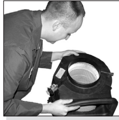
Inspect the engine air cleaner.
