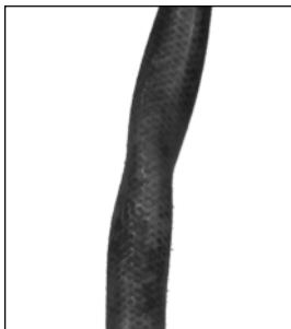
Partly collapsed inlet line shown.
