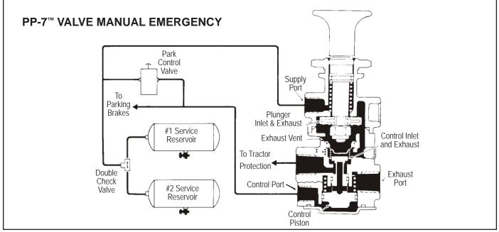
FIGURE 6 - PP-7<sup>™</sup> TRAILER SUPPLY VALVE MANUAL EMERGENCY
