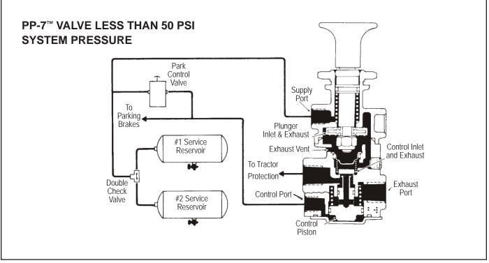
FIGURE 4 - PP-7<sup>™</sup> TRAILER SUPPLY VALVE LESS THAN 50 PSI SYSTEM PRESSURE
