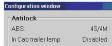
FIGURE 6 - CONFIGURATION WINDOW: IN-CAB TRAILER LAMP DISABLED
