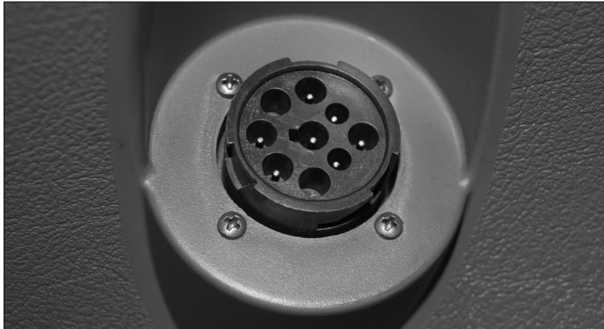
FIGURE 14 - TYPICAL VEHICLE DIAGNOSTIC CONNECTOR LOCATIONS (J1939)
