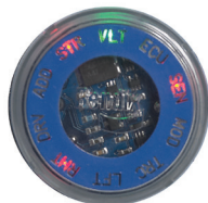
FIGURE 20 - DIAGNOSTIC TROUBLE CODES AS DISPLAYED ON THE BENDIX® RDU™ TOOL
