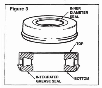
Be sure that the integrated grease seal on the bottom of the integral bearing is in contact with the axle beam.
