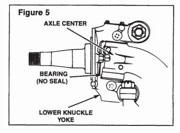
**IMPORTANT:** On front axles <u>without</u> thrust bearing seals, the bearing should always be installed in the axle with the closed retainer face up and the cage face (with the opening) downward.
