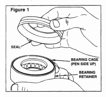
With the seal positioned on top of the thrust bearing, slide the bearing and seal assembly between the lower face of the axle center and the upper face of the lower knuckle yoke. See **Figure 2**.
