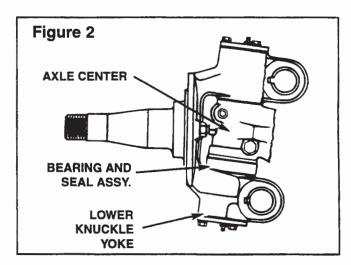
**IMPORTANT:** On axles with thrust bearing seals, the seal must always cover the opening between the bearing cage and retainer. Always install bearing and seal assembly in axle with seal on top.
