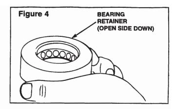
With the open side facing down, slide the bearing between the lower face of the axle center and the upper face of the lower knuckle yoke. See **Figure 5**.
